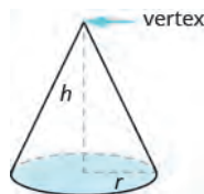
Figure 9.35 The height of a cone is the distance between its base and the vertex.
