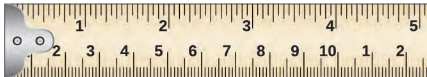
Figure 9.13 This tape measure measures inches along the top and centimeters along the bottom.
